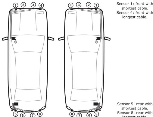
Sensor 1: front with shortest cable. Sensor 4: front with longest cable.
